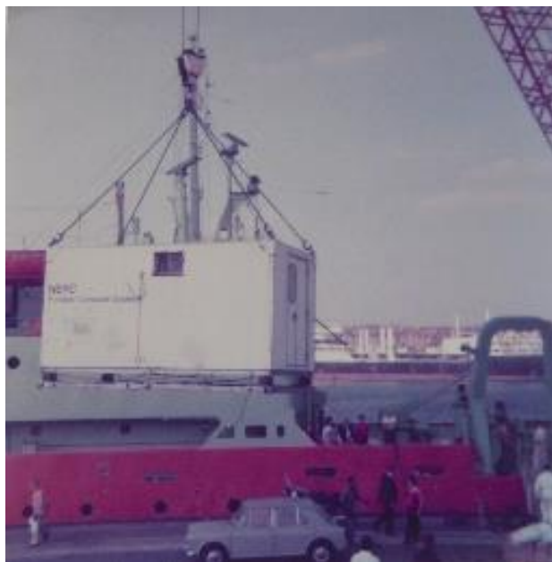
A containerised IBM 1130 computer system for data acquisition and processing being loaded into the forward hold of RRS Shackleton circa 1976.
